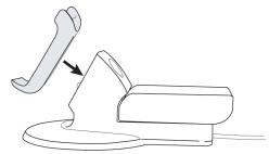
5. Slide the tabs downward in to the slots until the charging cradle is firmly in place.
